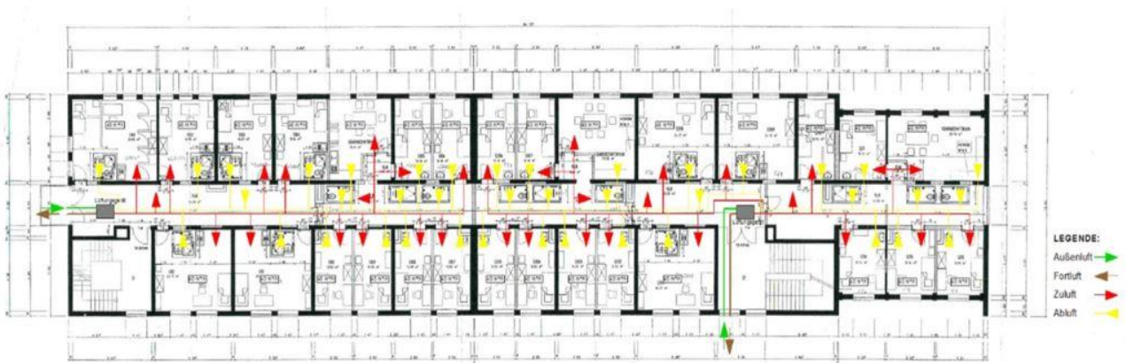
Figure A-2. Scheme of new mechanical ventilation system with fresh (green), inlet (red), outlet (brown) and exhaust air (yellow) applied in Bldg. 43.
