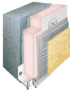
Figure A-4. Insulation composite system for Bldg. 42 with high resistant layers.
